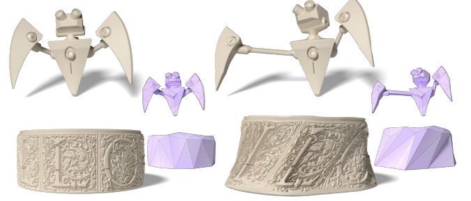
Fig. 24. Application in cage-based deformation. The top row illustrates a mechanical character, and the bottom row displays a high-resolution cylindrical relief. Left pair: Input meshes and automatically generated cages (purple) in their rest poses. Right pair: Deformed configurations achieved by manipulating the control cages. High-frequency surface details and structural integrity are maintained throughout the deformation process.
